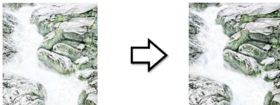
Figure 6-6 Original image is all in high gray level (Contrast Enhancement)
