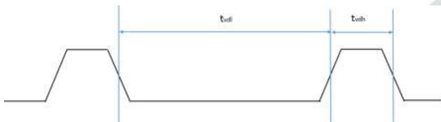
Figure 6-14 Tearing effect output signal mode 1
